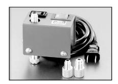
7. HFC refrigerant\_Electric gas leakage tester R32 refrigerant is often used for other mixed refrigerant (R410A, R404A, R407C etc.). Therefore, the usage of existing HFC detectors is possible, but in order to detect more accurately, we recommend to use detectors specially set and adjusted for R32 detection.
