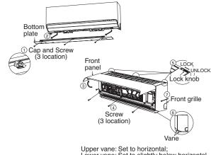
Upper vane: Set to horizontal; Lower vane: Set to slightly below horizontal
