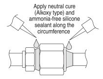
Neutral cure (Alkoxy type) & ammonia-free silicone sealant is only to be applied after pressure testing and cleaning up by following instructions of sealant, only to the outside of the connection. The aim is to prevent moisture from entering the connection joint and possible occurrence of freezing. Curing sealant will take some time. Make sure sealant will not peel off when wrapping the insulation.
