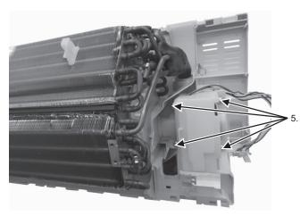
Remove 4 screws from fan motor cover.
