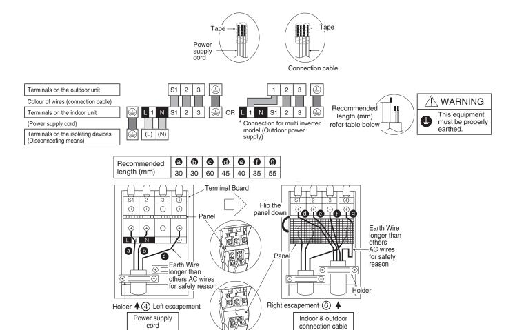
8 Secure firmly the power supply cord and connecting cable onto the control board with the holder. Do not overtighten holder screw, as this may damage the holder.
